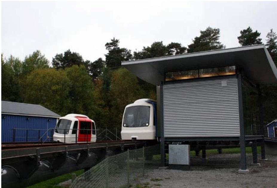
*Figure 1. In the photo you can see the first ever Podcar station with one car awaiting passengers, and with another car positioned on the main track.*
