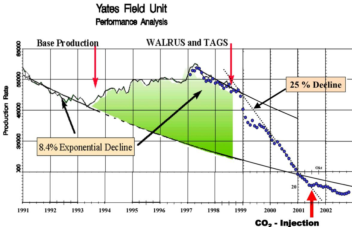
Figure 5: Yates field: total output increase was 40 million barrel with respect to total output since production start of 1.4 billion barrels (an increase of 3 percent). If the initial recovery rate was 20 percent, these EOR measures would have shifted the recovery rate to 20.6 percent. (RRC 2003)
