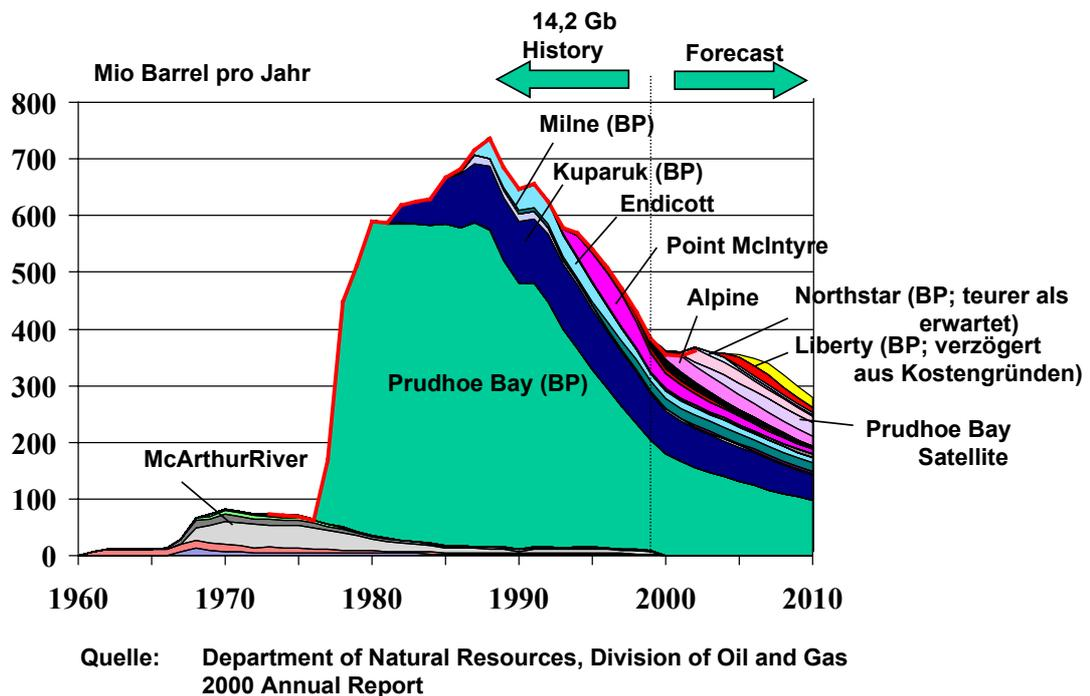
Figure 3: Field by field analysis of oil production in Alaska. The peaking oil production from Prudhoe Bay in 1989 set the scene for the unavoidable decline in production in the following years. Production from the small fields has succeeded in halting the decline at less than half the level of peak production, but this can last for only a few years, and at much higher costs than in the early production phase.
